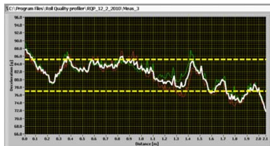
Figure 14. Reel hardness profile of 2100mm wide reel. (Mean hardness=81.3g \sigma=3.4g COV%=4.2%)
