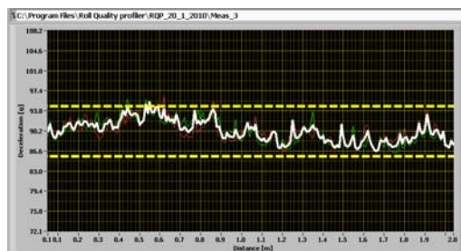
Figure 15. Reel hardness profile of 2000mm wide reel (Mean=90.4g \sigma=2.1g COV%=2.3%)
