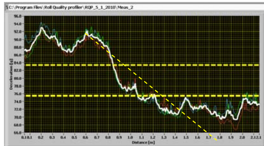
Figure 13. Reel hardness profile of 2100mm wide reel. Horizontal lines indicate the boundary of \pm 5\% from mean hardness. (Mean hardness = 79.5g \sigma=8.1g COV%=10.1%)
